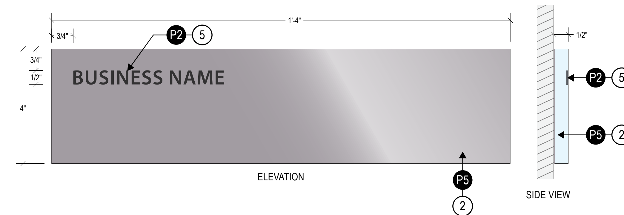
SILVER LEVEL PLAQUE - ELEVATION & SIDE VIEW (QTY. 7 SHOWN) SCALE: 6"=1'-0"
